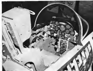
STUDENT'S COCKPIT (mockup) can be fitted with engine control pedestal status statement panel.
